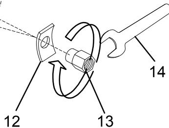
Do not tighten bolts until completely assembled
