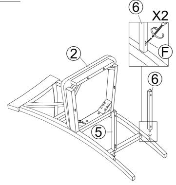
DO NOT TIGHTEN BOLTS UNTIL COMPLETELY ASSEMBLED.
