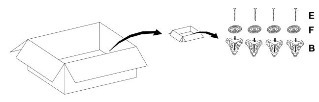
Step 2. Align the gasket onto the top of the legs and rotate to tighten it. Insert screws to the legs as shown in drawing and tighten it.
