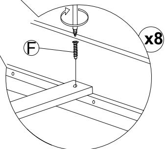
DO NOT TIGHTEN BOLTS UNTIL COMPLETELY ASSEMBLED.
