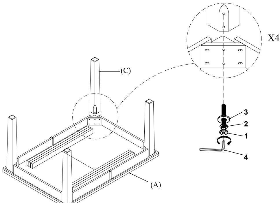
DO NOT TIGHTEN BOLTS UNTIL COMPLETELY ASSEMBLED.
