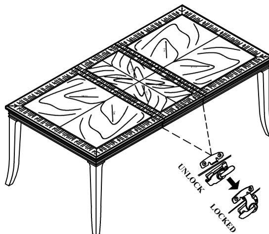
**DO NOT TIGHTEN BOLTS UNTIL COMPLETELY ASSEMBLED.**
